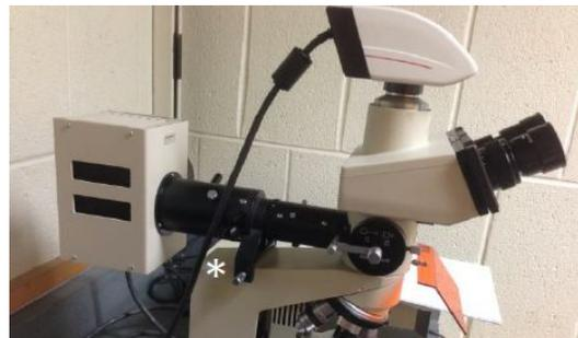
Do not look directly at the high-intensity light coming from the objective! Extended periods of exposure could damage your vision. Keep the orange screen in place to block out this light.
