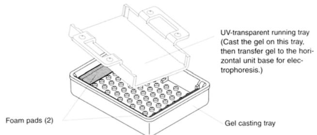
8. Use a bubble level to be sure the gel plate is flat; otherwise, you'll get a wedge-shaped gel.
