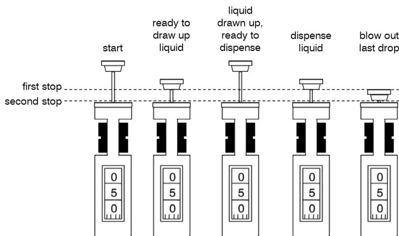
Follow the steps below carefully for best accuracy when working with micropipettors. Even small details like how deeply the tip goes into the liquid can make a difference with these small volumes. If something goes wrong or your pipettor doesn’t seem to be working, tell your instructor. Do not just throw it back in the drawer so that it affects someone else’s experiment.
