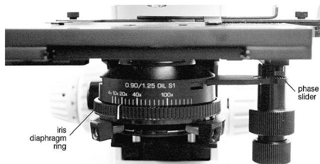
The DME microscopes have a 40× phase-contrast objective (*only* these lenses will work; don’t try to use phase at another magnification). The condensers of these microscopes have a slider (shown at left) allowing you to quickly convert between normal and phase-contrast mode. You can thus easily see what illumination works best for a particular specimen.
