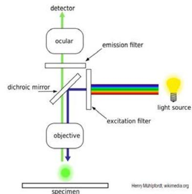
Fluorescence microscopes come with a variety of filters that can be used to obtain light of the correct excitation wavelength and to filter the emitted light that reaches your eye. To use a fluorescence microscope, you therefore need to know the excitation and emission wavelengths for the fluorescent molecule you are using and set the filters accordingly. The table at left gives excitation and emission wavelengths for some of the more common fluorophores.
