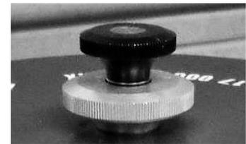
**Never, never attempt to run the centrifuge without either the lid or the running nut in place and properly tightened! If you have any question about your ability to use the centrifuge properly, check with a faculty member before starting the run.**
