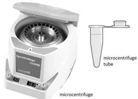
Microcentrifuges usually have only one rotor and may operate at a single, fixed speed (usually producing RCF of  $10,000$  to  $13,000 \times g$ ) or may have a variable speed. Some allow RCF to be set directly, while some require you to know the speed you want in RPM. Most have a timer to set a specific length for the centrifuge run; often, there is also a button that can be held down for a brief spin (e.g., a 5 s spin to bring droplets of liquid to the bottom of a tube).
